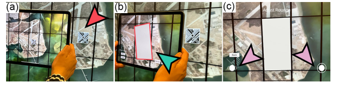
Figure 4: (a) Image marker, highlighted by the red arrow, used for initialization. (b) Misaligned mapping of the AR and LWD coordinate spaces, visualized using a reference plane. (c) The mapping can be fine-tuned using widgets, highlighted by the arrows.
