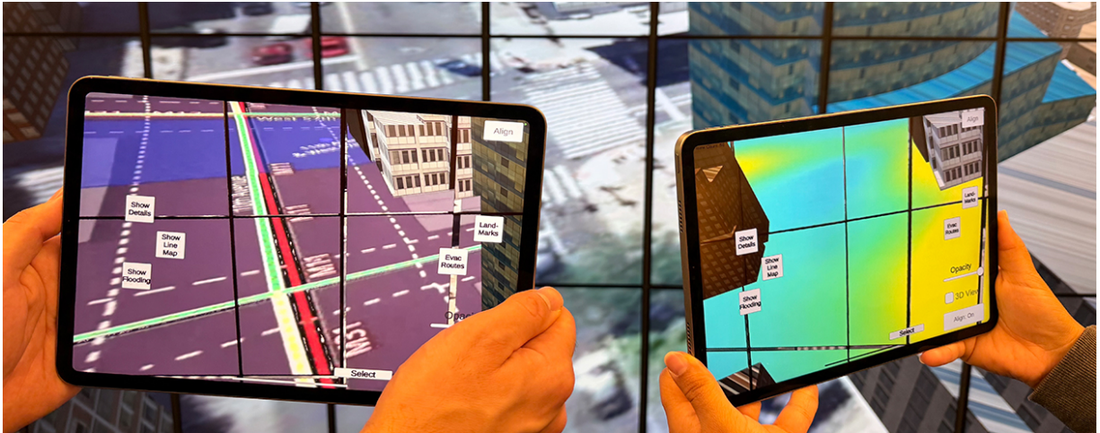
Figure 1: Two collaborators explore urban data using AuxiScope, which overlays AR visualizations on handheld tablets aligned with data displayed on a large wall display, enabling personalized, multi-user analysis without visual interference.
