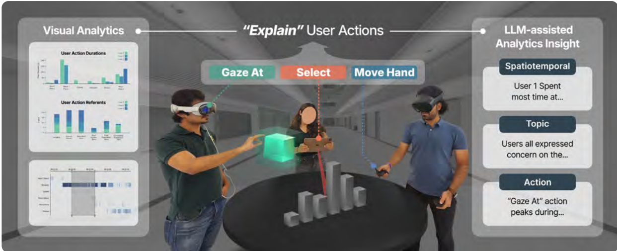
Fig. 1: Explainable XR provides a streamlined pipeline to record, visualize, and analyze users of an immersive session, facilitating researchers from various domains of expertise, to readily comprehend and study them. Our structured user data recording format captures users' actions (e.g., GazeAt, Move Hand, Select) and their contextual reasoning. Through our data analyzer and LLM-generated insights, we present base analytics interpretation of the users' action data on top of our visual analytics interface, and assist researchers to approach the analysis from multifaceted perspectives.
